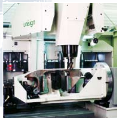
UNIVERS 6 with NC-table and tail stock centre for complete machining of bogey frame wheel carriers
