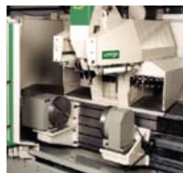
NC rotary table, designated as A-axis, with tail stock centre. Rotary table is located just outside the machine work area for maximum work area exploitation
