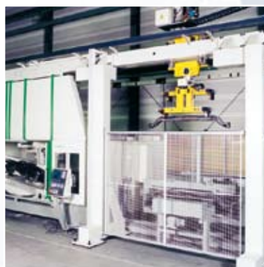
UNIVERS 6 as a flexible manufacturing system for complete machining of truck front axles
