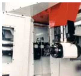
UNISIGN right angle head with automatic tool change from tool storage and automatic attachment procedures from pickup station (located just outside the working area)
