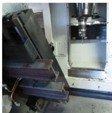
UNIVERS 6 as a flexible manufacturing system for complete machining of forklift mast channels
