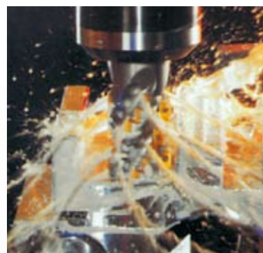
Coolant supply through the spindle and tool, including coolant filter unit with self-cleaning rotating filter
