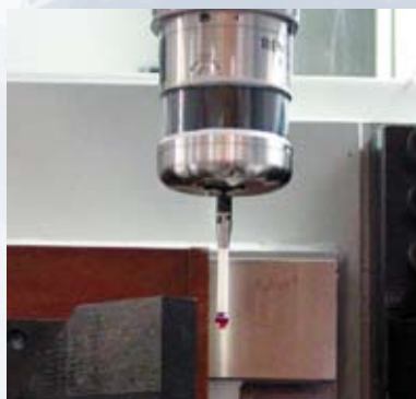
Wireless measuring probe for gauging / calibrating of reference points. The receiver is connected to the CNC control via an interface
