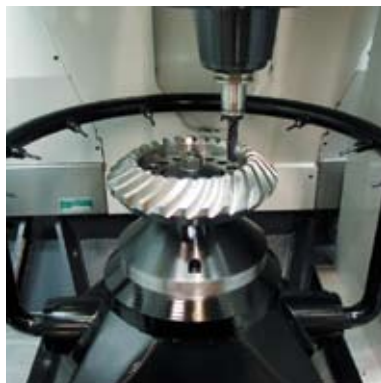
Component specific clamping fixture for machining of crown wheels
