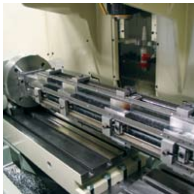
NC-table and tailstock centre with clamping cube, designated as A-axis
