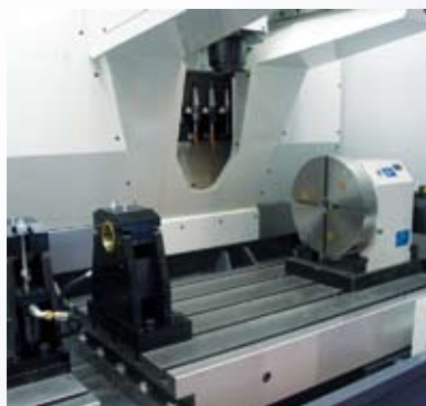
NC-Indexer designated as A-axis (also in pendulum mode)
