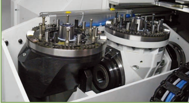
Photo: Spindle attachment pickup station with 6 positions
