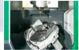
NC rotating & tilting table for 5-axes machining.
