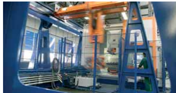
UNIPRO 5-S with rotating & tilting table and automatic loading robot for cylinder head machining.
