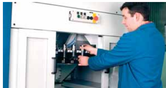
The tool loading bay allows the (un)loading of tools while the machine is in operation.
