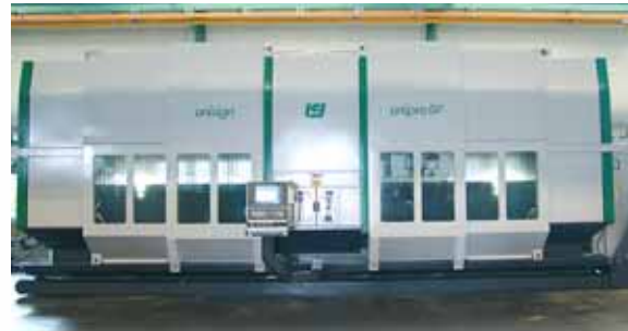
UNIPRO 5-P in extended execution with X = 2.000 mm for each work zone.
