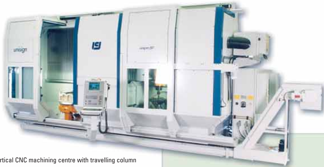
UNIPRO 5-P in standard execution with X = 1.000 mm for each work zone.
