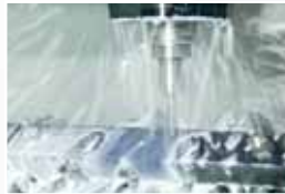
High pressure coolant supply centrally through the spindle and the tool.
