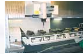
NC indexer with tailstock centre and clamping cradle.
