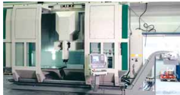
UNIPRO 5-L in standard configuration with X = 2.000 mm.
