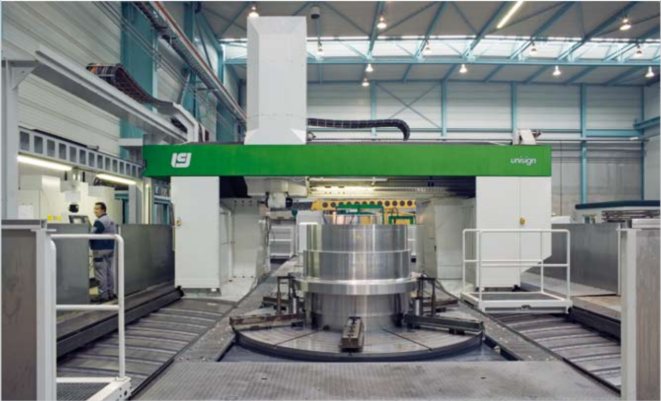
UNIPORT 8000 travelling bridge gantry machine
