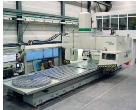
UNIPORT 6000 Travelling Bridge Machine with rotary table, designated as C-axis and fully integrated into the machine's base frame.
