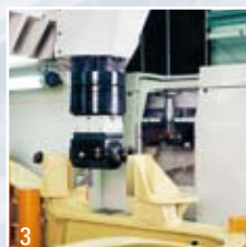
1. Right angle head for horizontal milling and drilling operations
