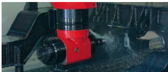
Large fabrications, such as rolling stock bogey frames and related components
