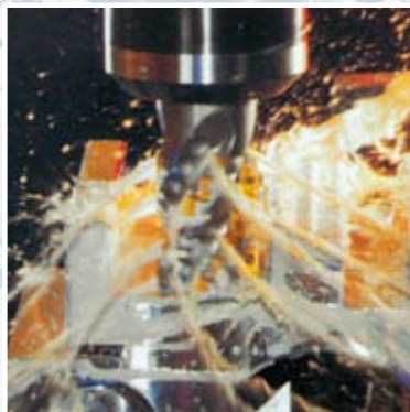
Coolant supply through the spindle and tool, including coolant filter unit with self-cleaning rotating filter
