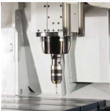
Wireless measuring probe for gauging / calibrating of reference points. The receiver is connected to the CNC control via an interface
