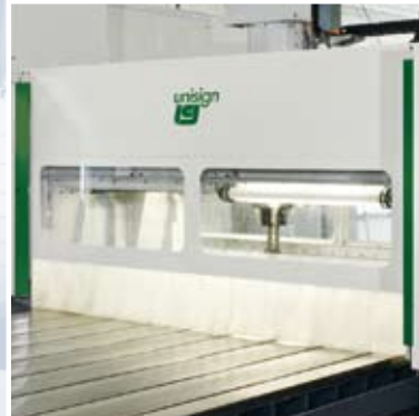
Safety panels adjustable in height via push-buttons on the control panel
