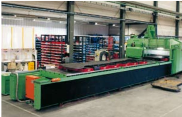
Production of side plates for earth moving equipment, with magnetic clamping plates
