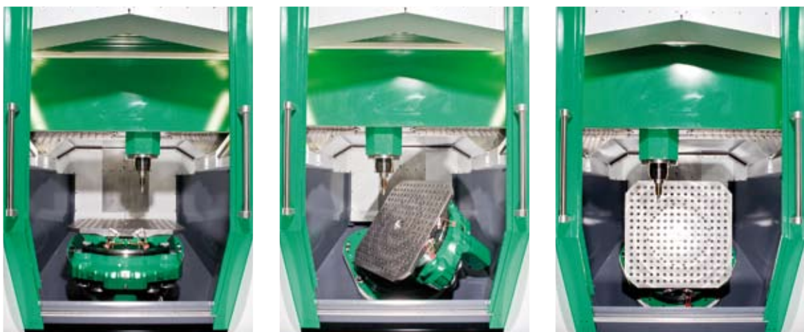
NC rotating and tilting table for 5-axes machining
