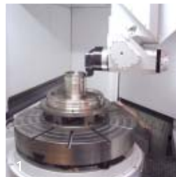
Spindle loaded adapter for turning tools (1 and 2)
